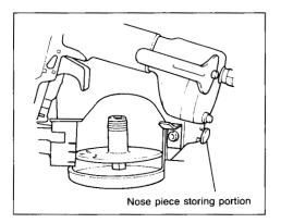
Attach the nose adapter to the contact arm (see right). When not in use, store the nose adapter at the rear of the tool to keep it from being lost.
